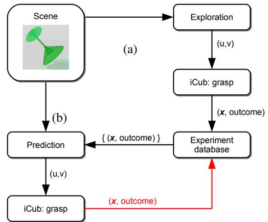
**Figure 3. System bootstrapping (a) and application (b) schemes of the presented system for a single image. The red arrow indicates the extended ability of on-line learning.**
