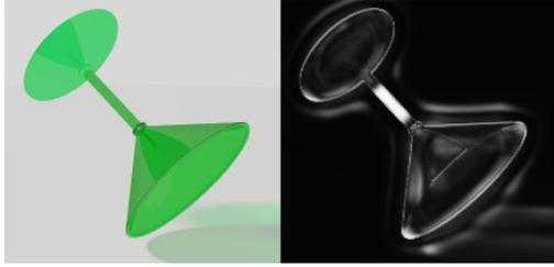
**Figure 2. The predicted probability map for an upside down Martini glass. The brighter an area is in the right image, the higher is the probability for a successful grasp.**
